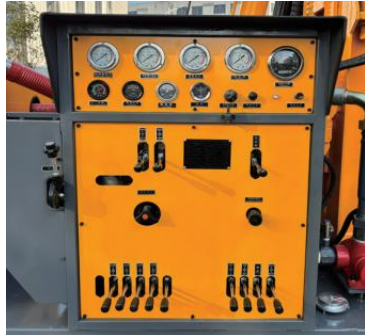
操作阀面板 Operating valve panel
