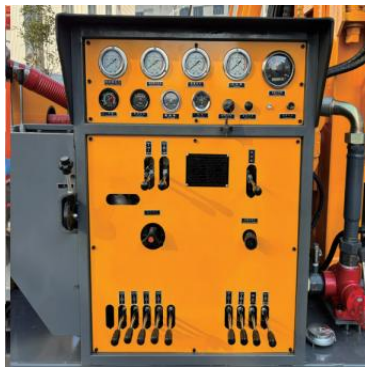
操作阀面板 Operating valve panel
