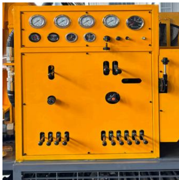
操作阀面板 Operating valve panel
